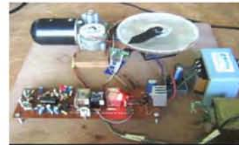
Fig. 17 Photo Showing 20 kVA, Automatic Voltage Stabilizer Control System at Normal Condition
